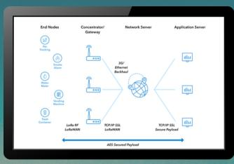
Telemetry2U employs LoRaWAN to send data to our cloud servers. LoRaWAN is a cutting-edge, wireless technology that's fast becoming the go-to protocol used to connect sensors and devices to the 'Internet of Things'.
