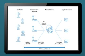
Telemetry2U employs LoRaWAN technology to transfer data between the real world and our cloud based IoT platform. LoRaWAN is a long-range, wireless network that's fast becoming the go-to protocol used to connect devices and equipment to the 'Internet of Things'.
